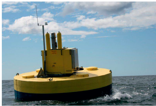
Fig. 1. Fred Olsens Wave Energy Converter BOLT ® located outside Risør, Norway
