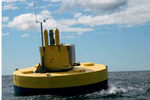
Figure 3: FO's Wave Energy Converter Bolt , located outside Risør, Norway has been in operation since June 2009.
