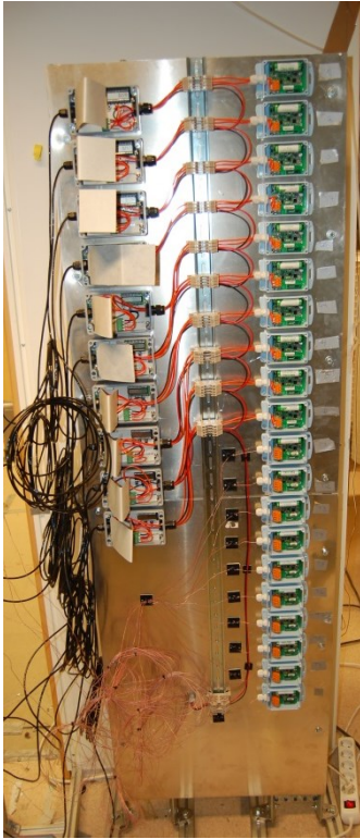
Figure 70: The setup for the transducers and the sensors for the velocities and temperatures in the aperture.
