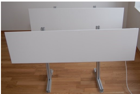
Figure 72: The panel heaters.
