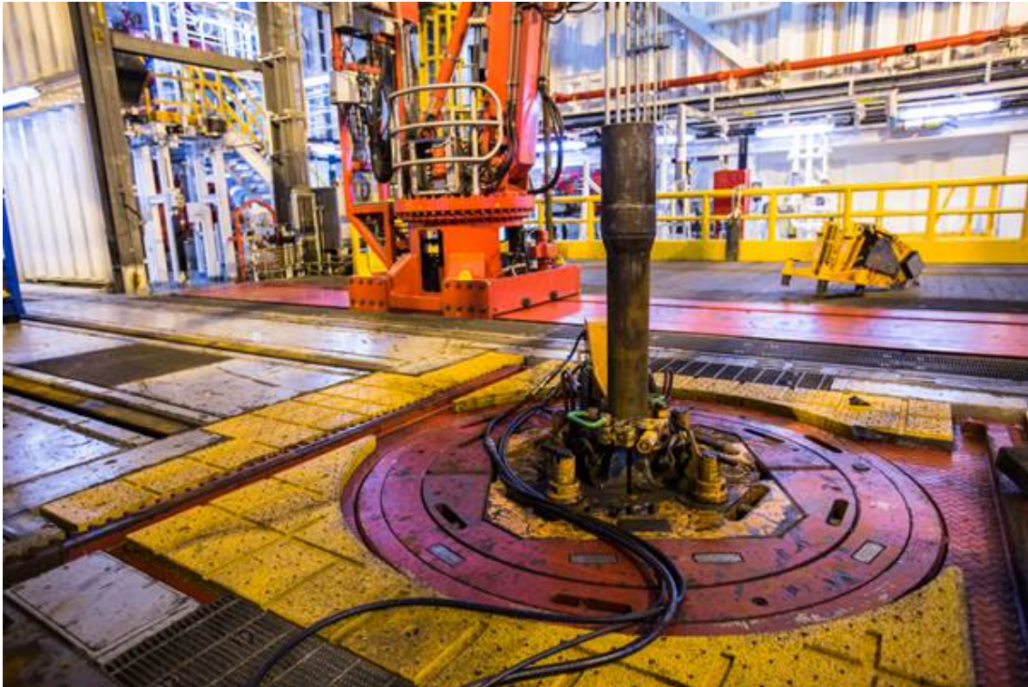
Figure 3.17: Well center, at the base of the drill floor. Credit: Vegard Haugland, MHWirth AS, Haugland (2015)
