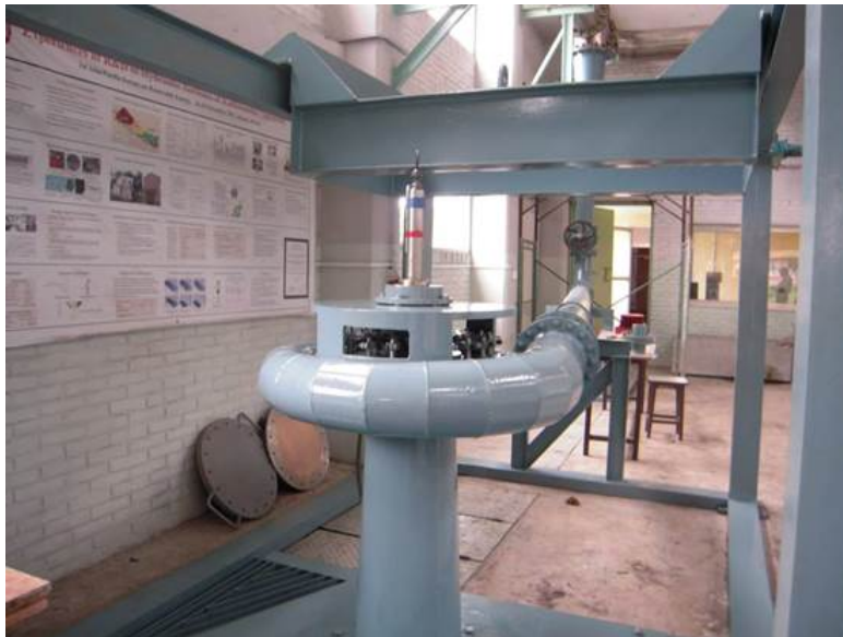
FIGURE 2.6: The simplified turbine test rig at TTL [10].
