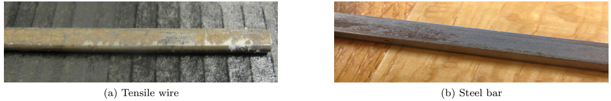
Figure 3: The tensile wire was cut from the same test pipe in the full scale testing. The steel bar was separately manufactured for achieving full contact.
