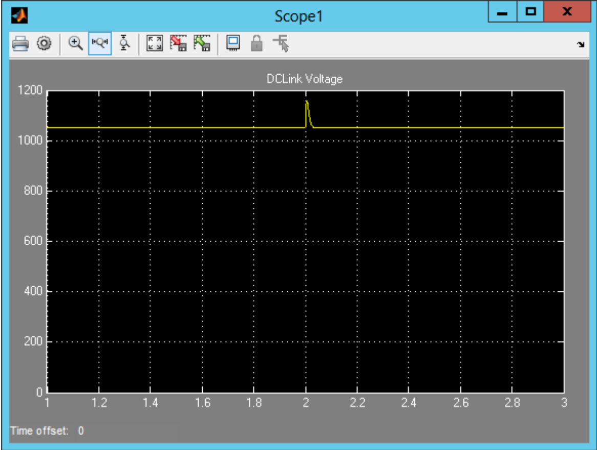
Figure 26 – Voltage over the capacitor in load converter.
