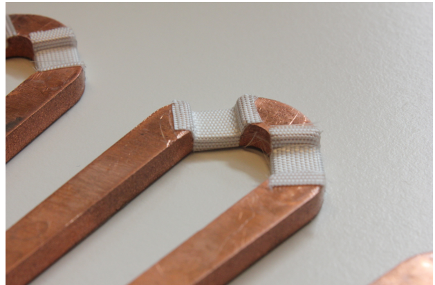
Fig. 47: The insulation method, two tape layers in an X
