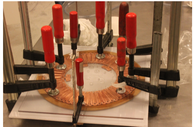
Fig. 50: A number of vices is used to compress the mold to leave a thin epoxy layer on the stator
