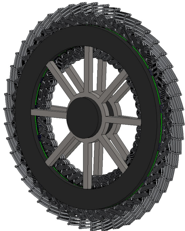
Fig. 12: 3-layer, dual leveled, lap windinded, slotted internal stator AFPM,
