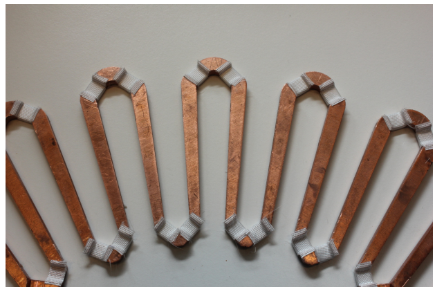
Fig. 48: Section of a fully insulated winding
