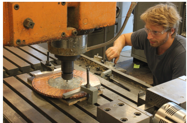
Fig. 51: Milling the shaft hole, where the center of the geometry is found
