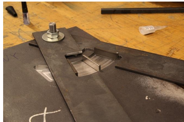
Figure 29: Jig for assembling magnets.
