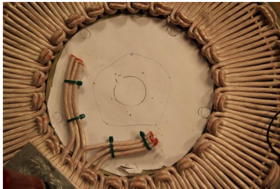
Figure 13: The end turns of the top phase is always crossing on top.
