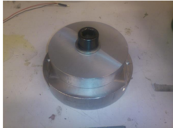
Figure 28: Finished with a powerful top part to hold the magnets in place.
