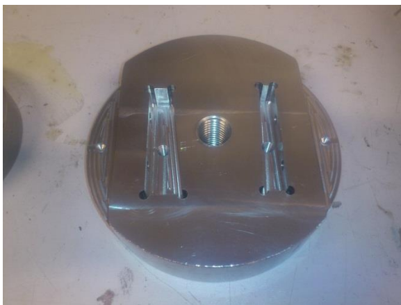
Figure 27: Mold to glue magnets together.
