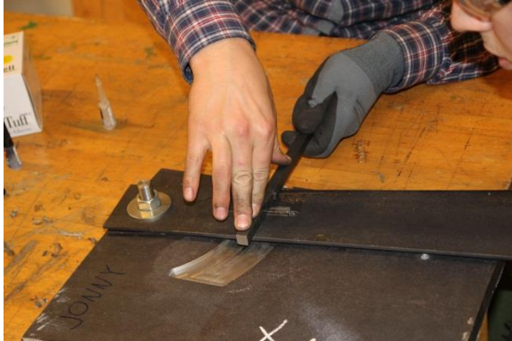
Figure 30: Steel in all directions was the only way to keep the magnets in place.
