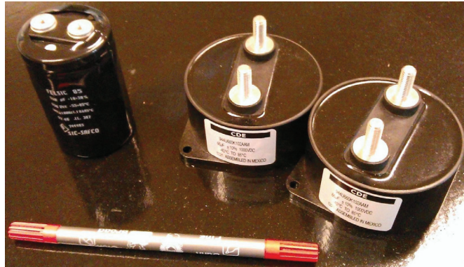
Figure 10.1.1: Comparison of volume between electrolytic and film capacitors. Left: Electrolytic, 330\mu\text{F} , 630VDC. Right: Film, 2\cdot66\mu\text{F} 1000VDC.
