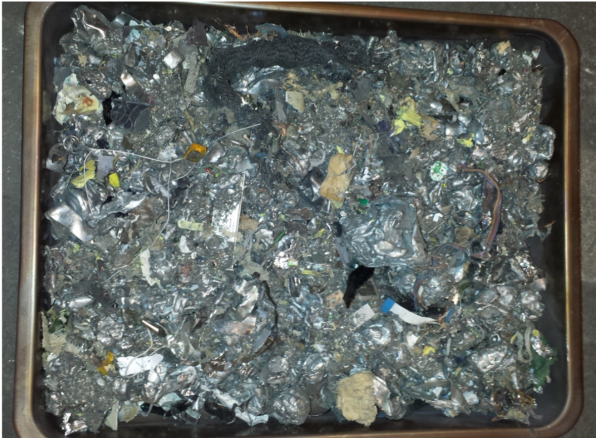
Figure 4-10 Tray with scrap from Input 2c MET-2 after demagnetization. Most of the plastic parts were slightly deformed, but remained whole. The trays, of size 40x32 cm, suffered slight deformation, but were reused without trouble.
