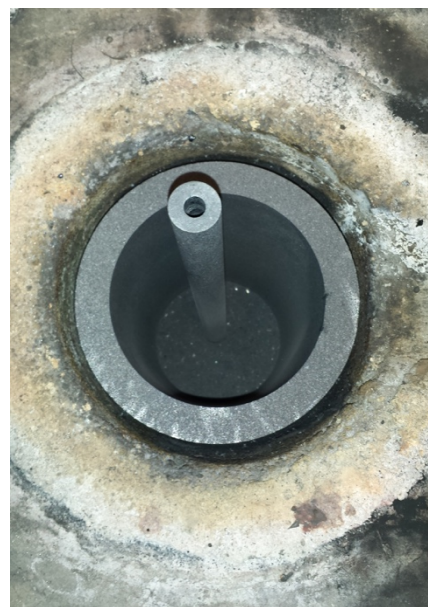
Figure 4-15 Setup of large-scale experiments. The thermocouple was placed inside the graphite tube.
