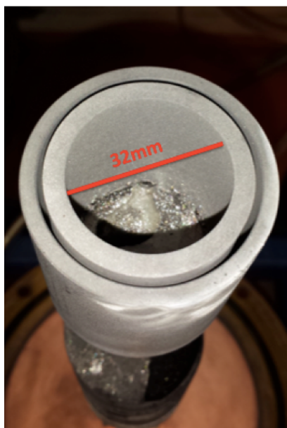
Figure 4-13 Inner crucible placed inside outer crucible and filled with material.
