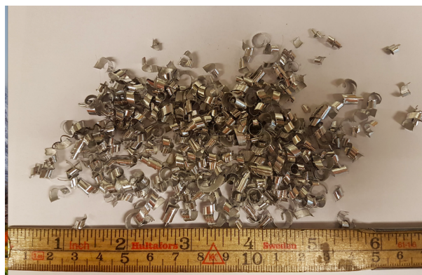
Figure 3.6.1: Machined granulates of the engine block. The granulates of the two Al-Si alloys were nearly identical.
