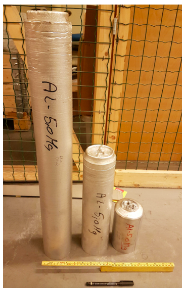
Figure 3.1.1: Picture of the Al-Mg billets before homogenisation and extrusion.
