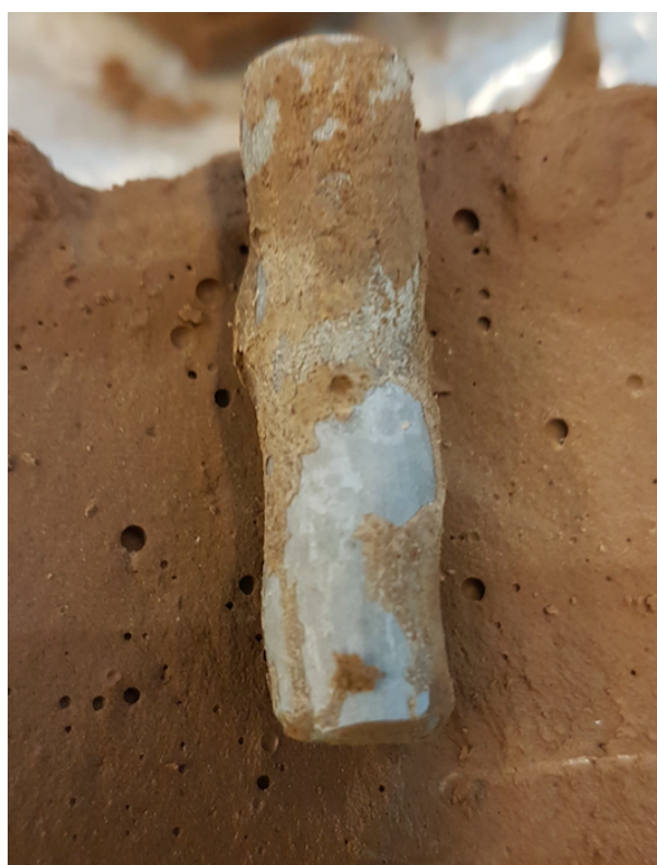
Figure 5.4.1: The figure shows a sample from one of the hydrogen evolution trials where the hardened cement sample is split in two after 14 days in order to observe the aluminium surface after corrosion.
