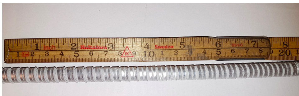
(b) The profile of the engine block material. The extrusion direction is to the left in this picture.
