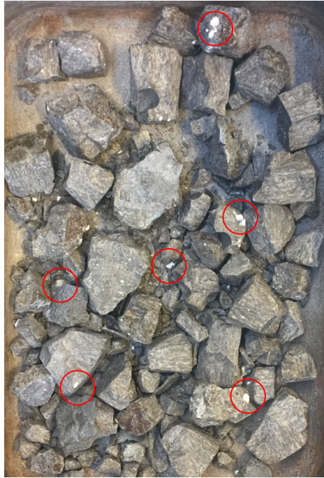
Figure 5.12: Synthetic slag after crushing in agate mortar. Red circles indicate areas containing CaO pieces
