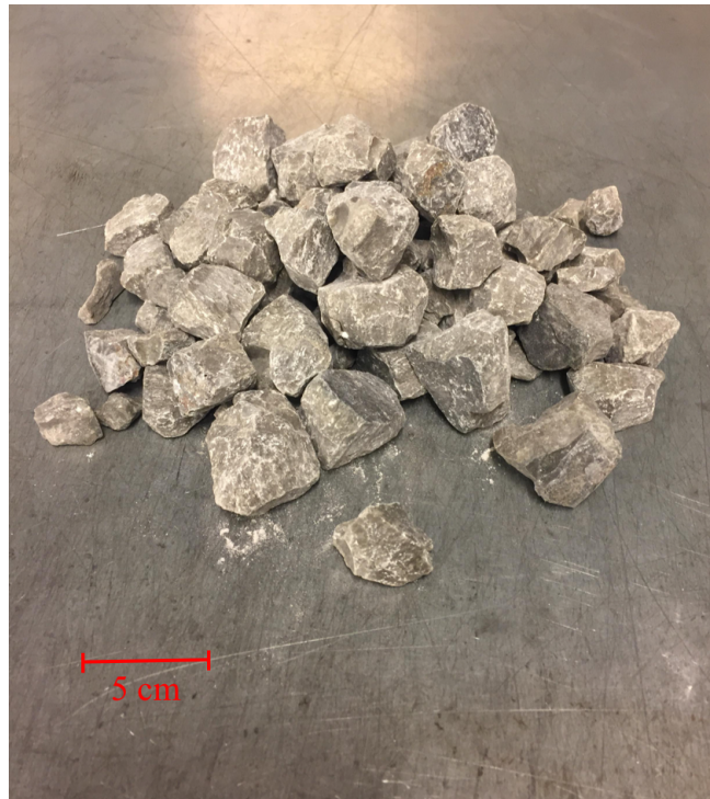
Figure 3.5: Produced slag used as the silicon source
