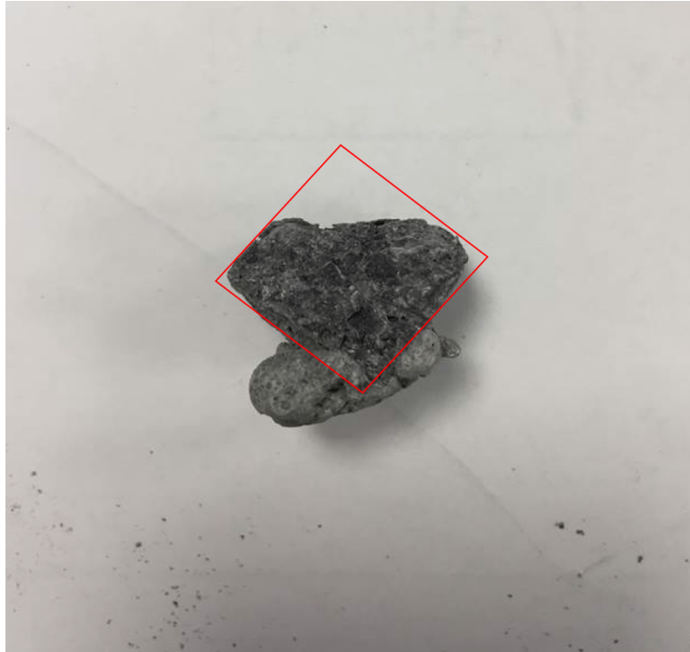
Figure 5.2: Extracted UBC piece after coalescence experiment seen from above. The red square indicates the original form of the material
