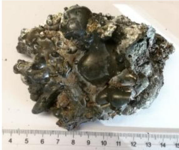
Figure 4.11: Slag sample from the front of the runner collected after tapping session 2496 (slag sample 3).
