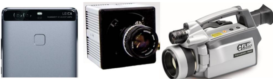
Figure A.2: From left to right: The phone camera, high speed camera, and infrared camera used in the experiments.
