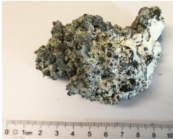
Figure 4.10: Slag sample from one of the sides of the runner collected after tapping session 2496 (slag sample 2).
