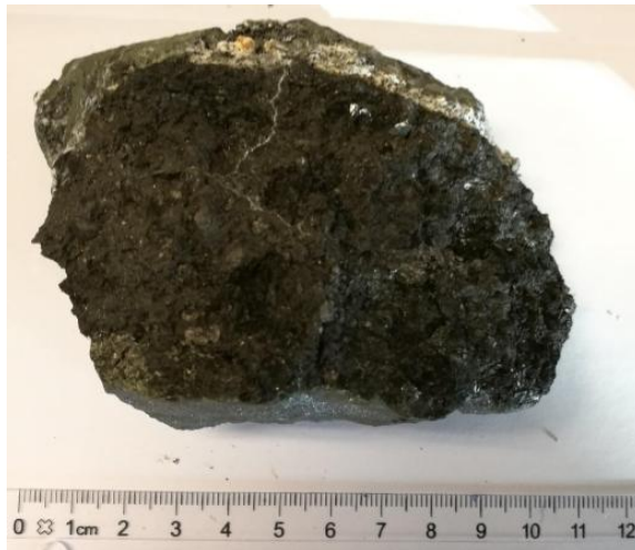
Figure 4.12: Slag sample from the bottom of the runner collected after tapping session 2496 (slag sample 4).
