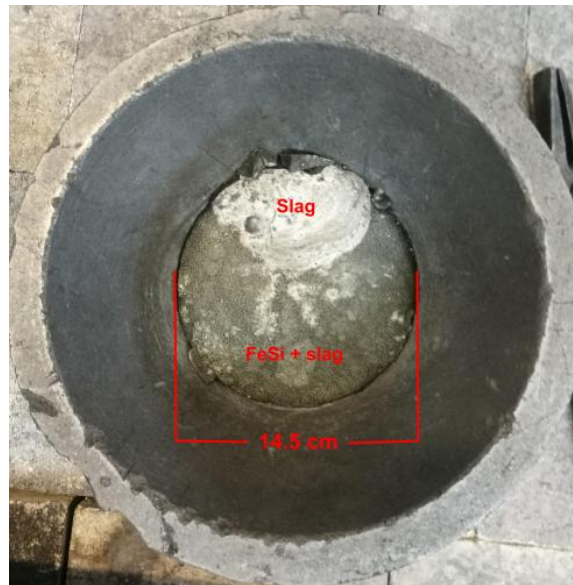
Figure A.7: The solidified slag and FeSi after experiment 1.
