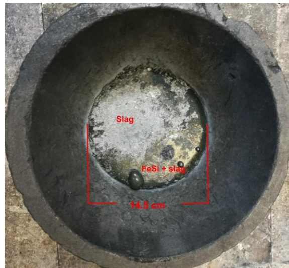
Figure A.10: The solidified slag and FeSi after experiment 2.
