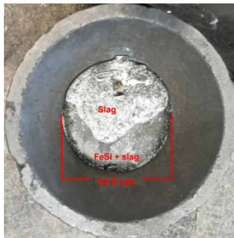
Figure A.13: The solidified slag and FeSi after experiment 3.
