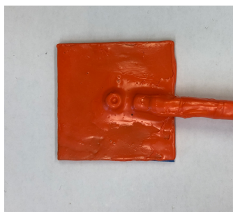
Figure 3.5: Preparation of the samples involved in OCP and galvanic corrosion experiment: The sample was connected to a wire by a cable shoe and a screw. The exposed area was covered with masking tape to prevent spill of the coating. The backside and edges in addition to the wire were coated by Micro lacquer (steel samples), bee wax (sacrificial anode and the aluminium alloys).
