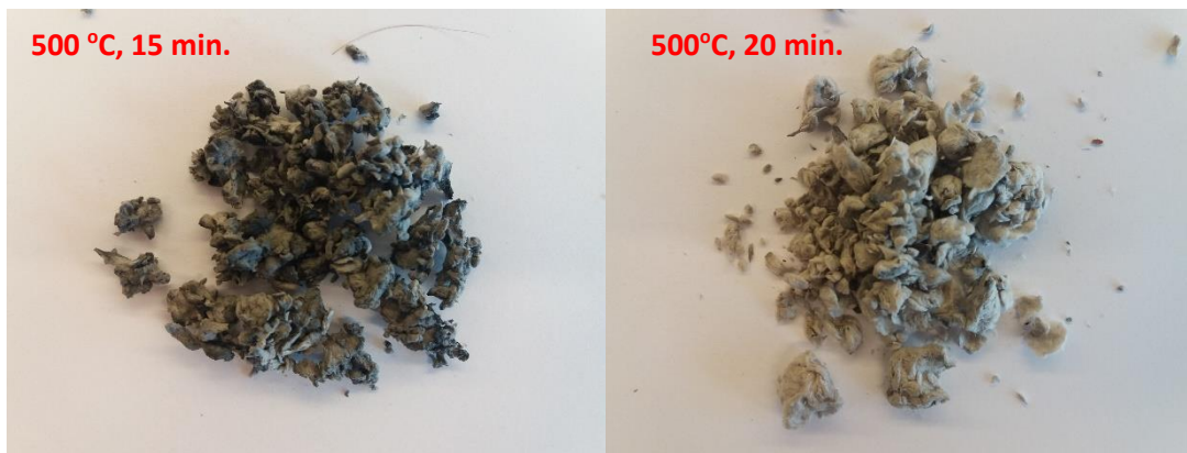
Figure 45 c-d: Glass wool waste exposed to 500 °C for c) 15 min. and d) 20 minutes
