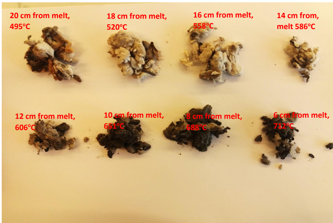
Figure 65: waste dug out from the crucible. The sample at the top left corner was closest to the top, and the bottom right closer to the melt
