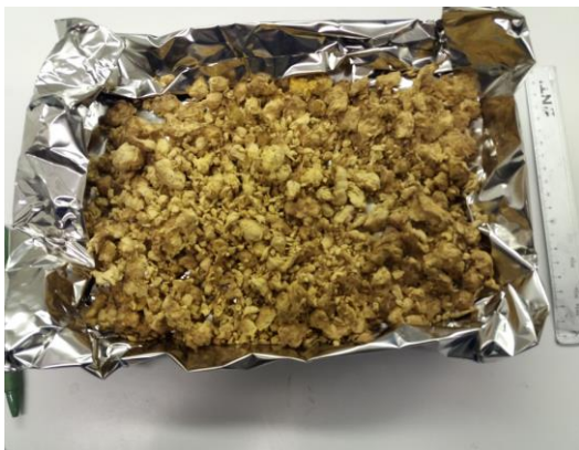
Figure 7: Glass wool waste after being dried in an oven for 48 hours.
