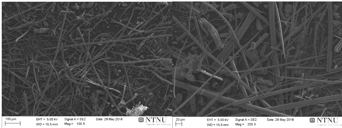
Figure 49 a-b: Sample after heating at 500°C for 3 minutes, at a) 100x and b) 200x
