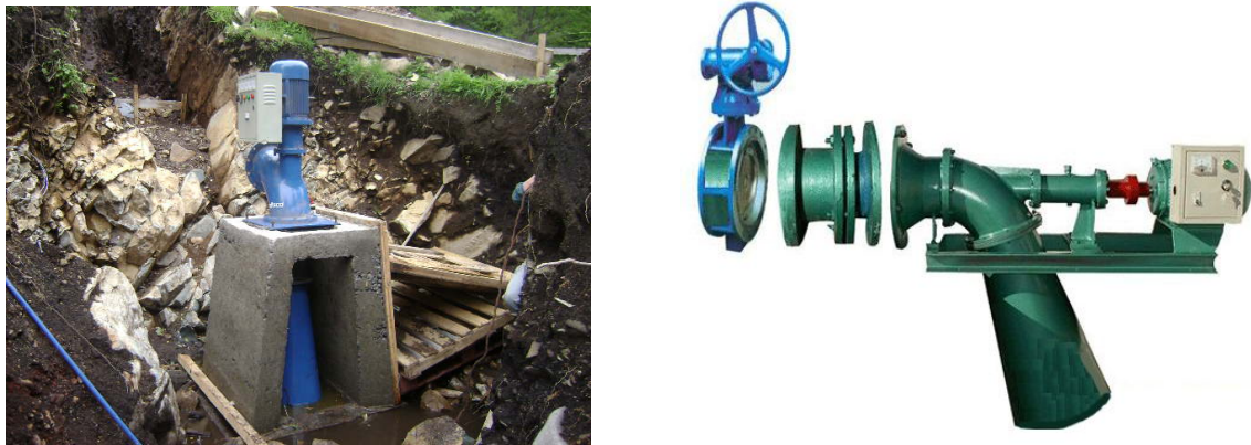
FIGURE 7.3: Medium Head Water Turbines Left: “front axle stretch” and vertical axis [26] Right: “level rear axle stretch form” [27]
