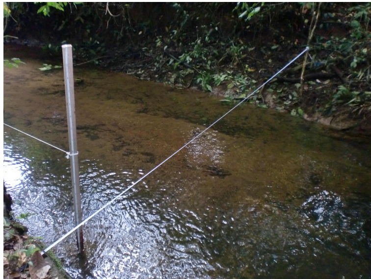
FIGURE 6.7: Gauging station in State Creek
