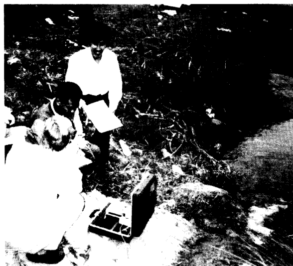
Photo 2.3.1 One suitable method of flow measurement for correlation is the salt dilution method. This requires a conductivity meter and a weighed quantity of salt.
