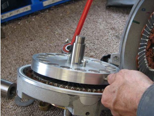
Technique for removing rotor showing jacking screws
