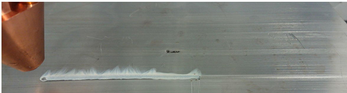
Figure 5-10: Image of the last run by moving laser on profile. The laser burned through the surface oxide layer and the material started to melt.
