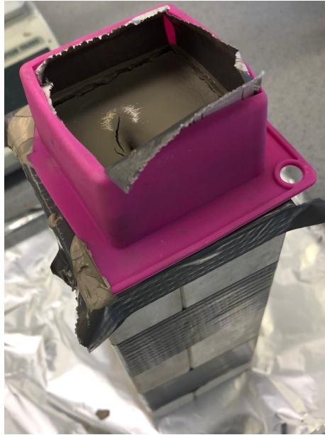
Figure 3-4 Image of the assembled mould with casted slip. The two mould parts are held together with duct tape and a silicone reservoir (pink) hold the excess slip.
