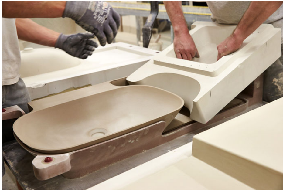
Figure 2-6 Demoulding of slip casted sanitary ware in a Roca factory [37]
