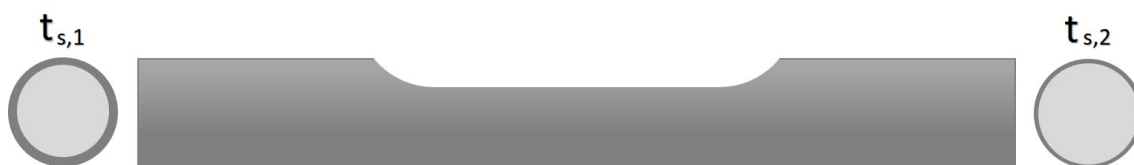
Figure 3.13: Illustration of how the thickness of the sleeve varies in one tensile specimen. t_{s,1} is the sleeve thickness on one side and t_{s,2} is the sleeve thickness of the other side.
