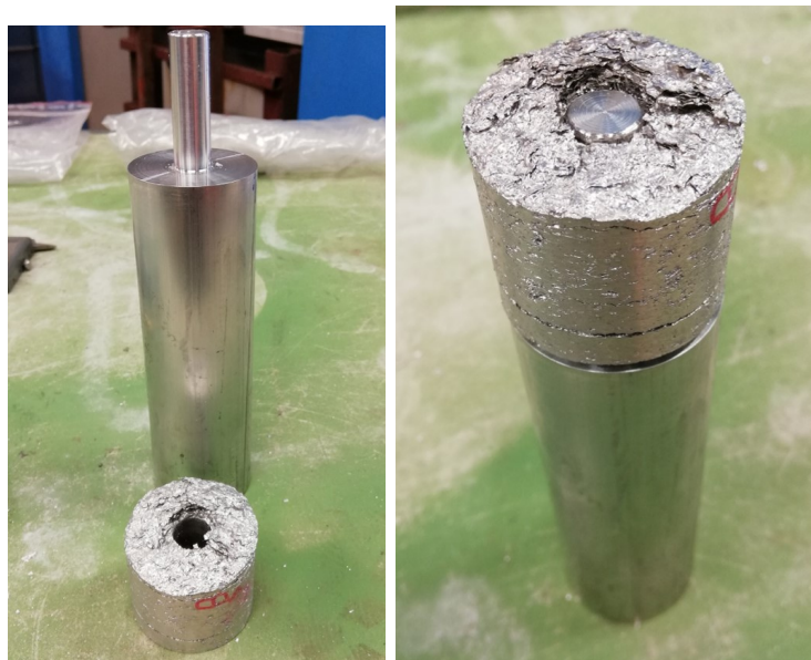
(a) Machined core and (b) Sleeve billet on top of the sleeve billets. core billet.
