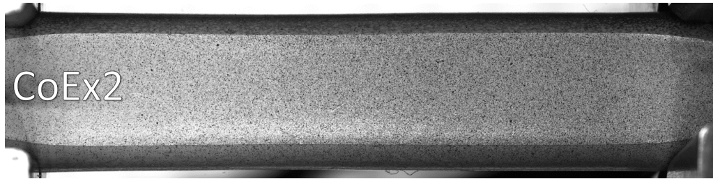
(b) Image taken of a specimen from CoEx2-Sc with a sleeve thickness of 117\ \mu\text{m} being subjected to 199\ \text{MPa} and 0.2 strain.
