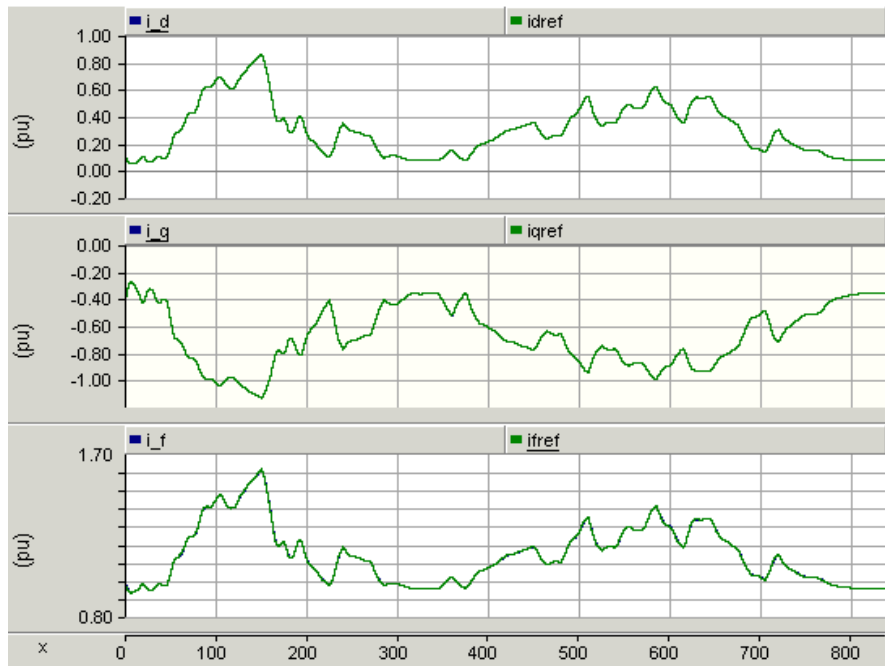
Figure 102: Generator operation: D-axis current, q-axis current and field current with references
