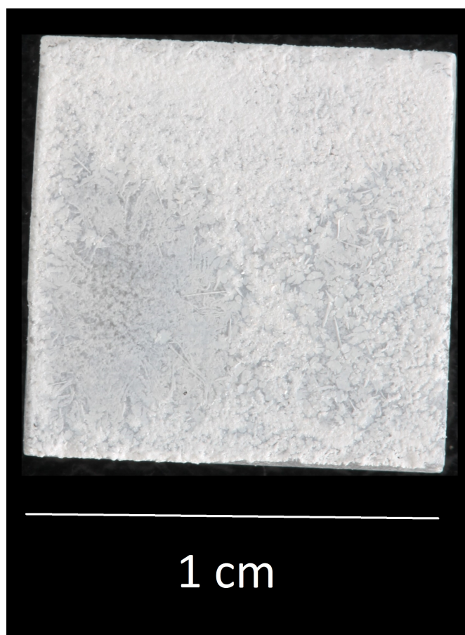
Figure 42: Silica crucible sample coated with Ba(OH) 2 solution
