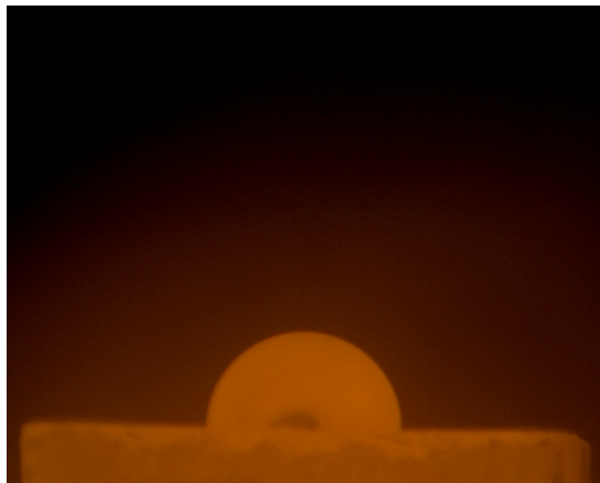
(a) No heat treatment, \theta = 88.08^\circ
