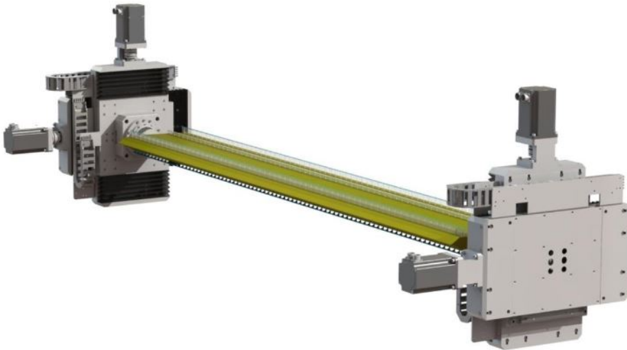
Figure 4.1: Basic working principle of a forced vibration rig: Bridge deck section model fixed between two internally connected actuators. (Siedziako, 2018)
