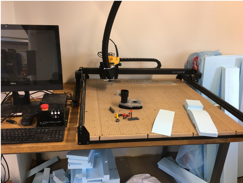
Figure 3.11: The X-Carve milling rig used for making the model.
