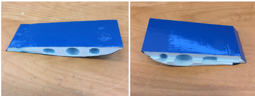
(a) First test and foil applied with heat gun at 600 degrees Celsius. (b) Second test and foil applied with heat gun at 400 degrees Celsius.
