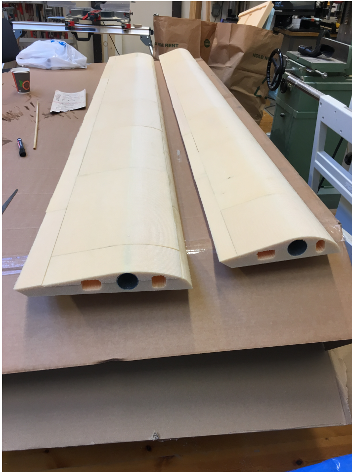
Figure 3.16: Twin deck model after gluing.
