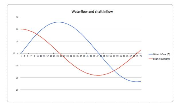
Figure shows the water inflow Q and the water level in the shaft (m) in ratio to seconds.
