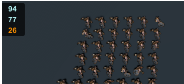
Figure 4.3: FPS counter for Unity showing max, average and lowest fps based on the 60 last measurements
