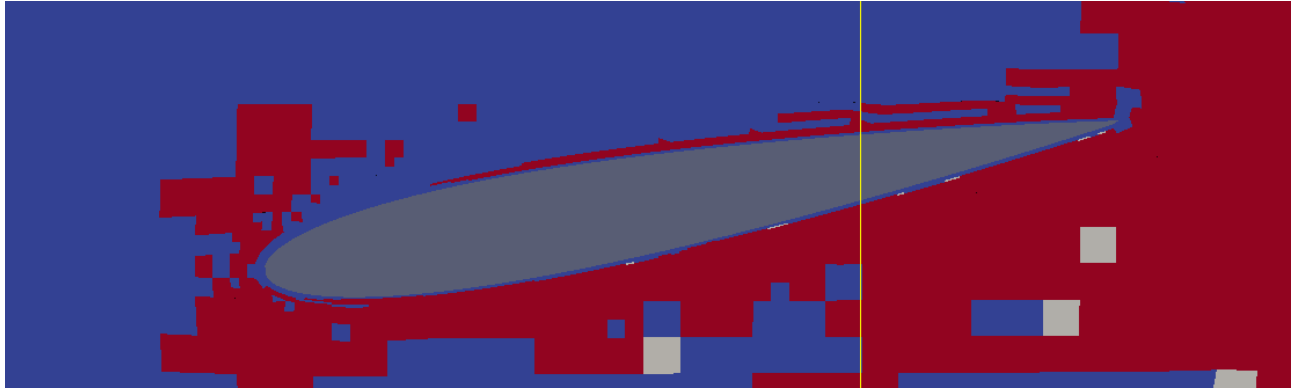
Illustration 32: RANS/LES distribution for DES of NACA-0012 foil at ten degrees angle of attack on "medium" grid.
