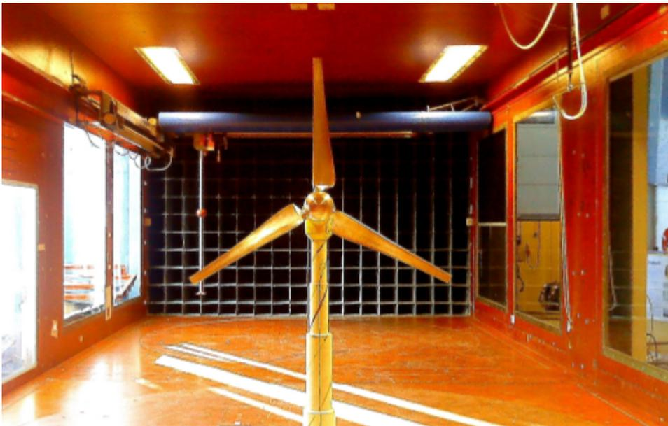
**Figure 10:** A picture of the wind tunnel with the model turbine at NTNU from "Blind test 1" [9].
