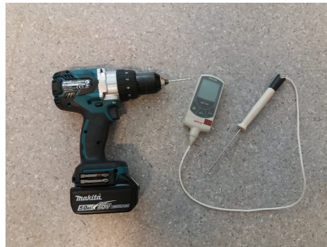
Figure 3.9: The thermometer and the drill bit is used for ice temperature measurements. The tip of the thermometer is stuck into a hole in the ice made by the drill bit.
