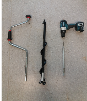
Figure 3.3: Ice drill with two types of handle mechanisms. Left: manual handle, middle: ice drill, right: grip for battery drill.
