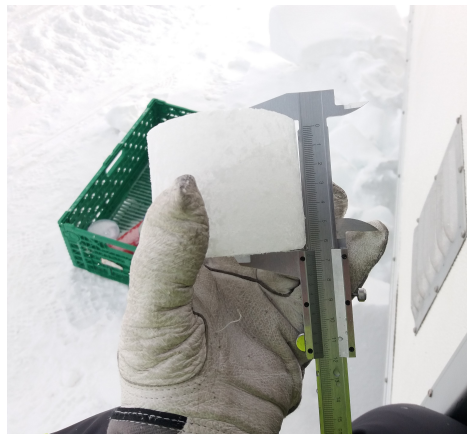
Figure 3.12: Caliper used to measure the length of the ice cores after the ends are cut.
