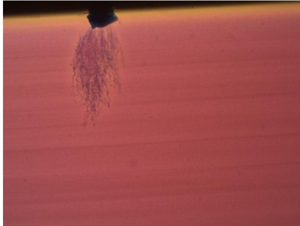
Figure 6.1. Impurity and resulting vented water tree from upper semiconductor.
