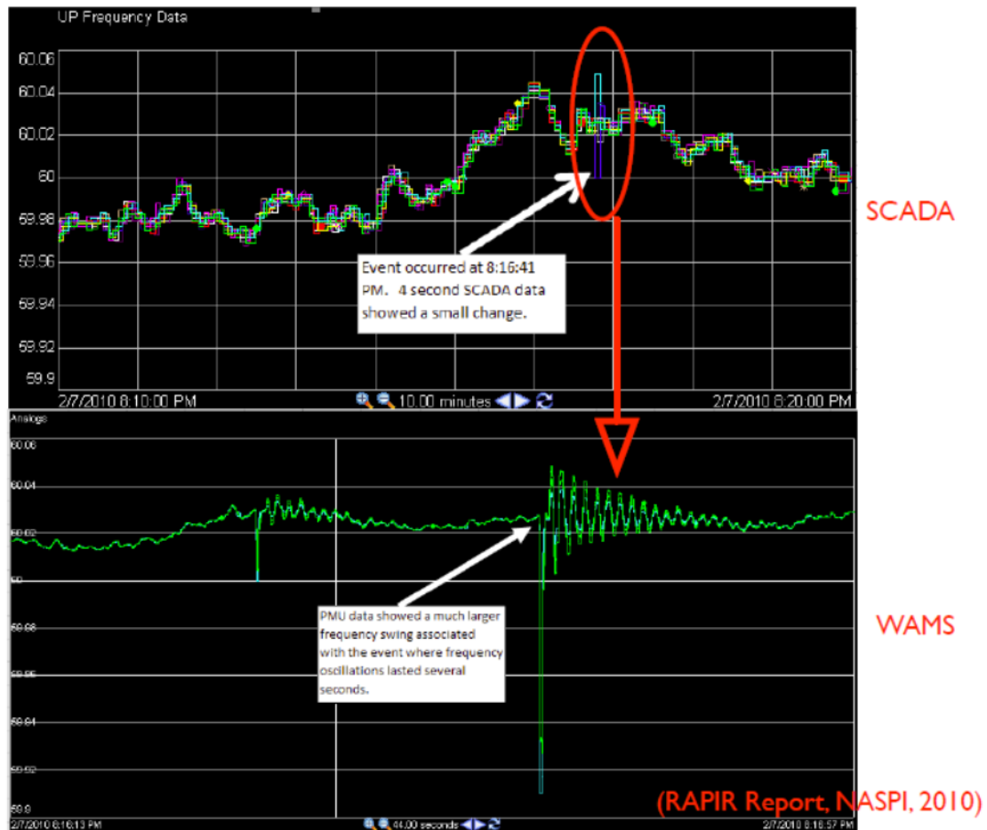
Figur 5 - Sensor system: SCADA vs. WAMS. Kilde: Vanfretti, 2011[12].
