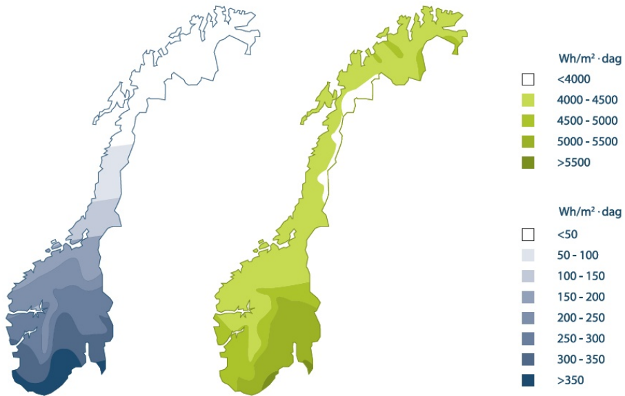
Figure 3.1.4: Solar irradiation map of Norway on a horizontal in January and July, measured in \text{Wh/m}^2 \text{ day} [17]
