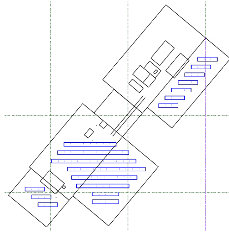
Figure 3.3.13: The modules on the roof drawn with rectangles
