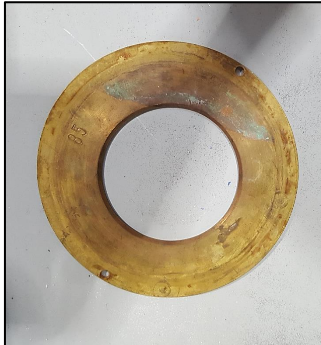
Figure 4.7: The orifice plate fitted between the two sections, where pressure drop is measured and the airflow rate is accurately calculated.
