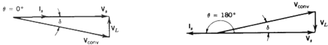
Figure 3-4 Rectifier mode (left) and Inverter mode (right) of operation at unity power factor
