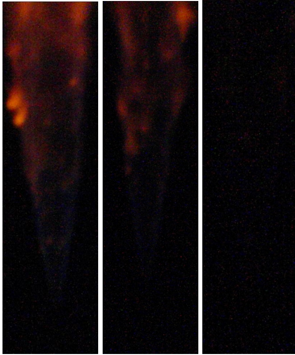
Figure 5.4.: Direct imaging of hydrogen jet flame with shutter times of 8 ms, 5 ms and 1 ms from left to right showing that direct imaging does not work [North, 2010].
