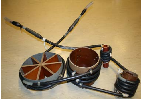
Figure 3. A cable bent around pipes of four different diameters.
