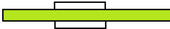
Figure 4-3 Strip line connection, the copper traces are white while the insulating PCB is green
