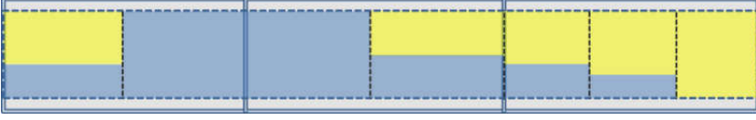
Figure 2.4. Example where fluid and structural discretization do not match
