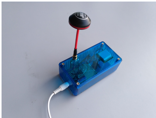
Figure 6.4: Prototype of the time beacon with embedded GPS module and 5.8GHz transmitter
