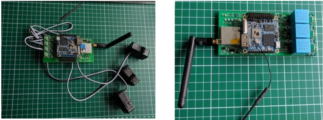
Figure 6.5: LVSensors, current sensor on the left and voltage sensor on the right
