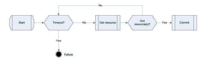
Figure 7 Resource reservation with timeout and failure
