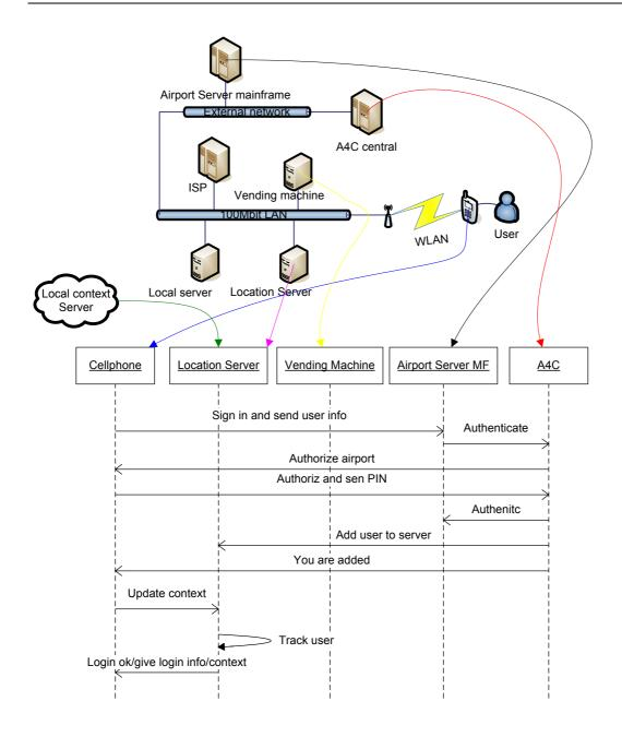
Figure 23 MSC of the context applet located in the Location server (device 2)
