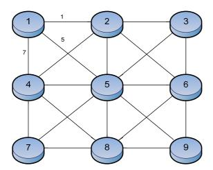
Figure 11 Step 1 of Dijkstra's algorithm
