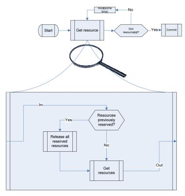
Figure 6 Internals of the "get resource-block" from Figure 5
