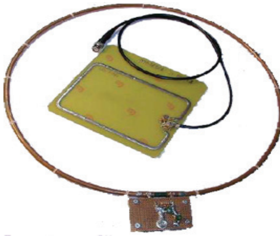
Figure 19: PCB and Copper-Tube antennas used by Kirschenbaum and Wool [20]
