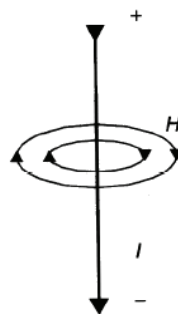
Figure 5: Lines of magnetic flux around current-carrying conductor [5]
