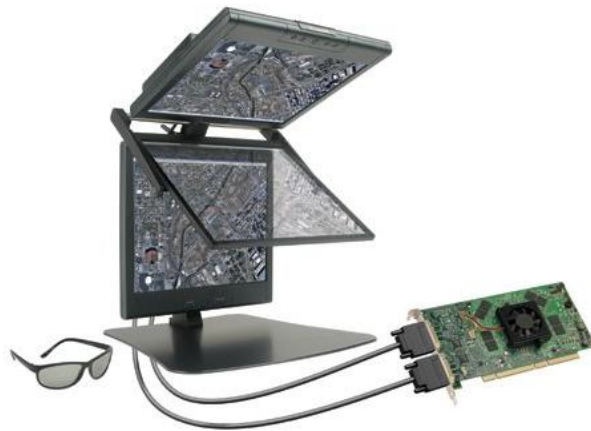
Figure 22: Planar SD170, Matrox Parhelia Precision and polarized glasses [48]
