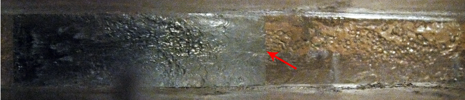
Figure 5.15: Liquid film pattern over the profile section. The red arrow indicating the trailing edge.
