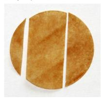
The resistance readings gave a value of at least  $200G\Omega$  for all readings
