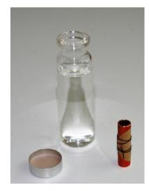
Figure 4.3: Example of created sample ready for copper sulphide growth. The glass tube contains corrosive Nytro10X oil
