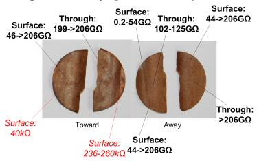
Figure A.33: Sample grown for fourteen days. Red and italic - Multimeter, Black and bold - Megger at 200V
