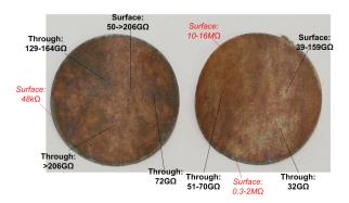
Figure 5.3: Two paper samples with copper sulphide contamination grown for seven days. Only the side that faced toward the copper during growth is shown.
