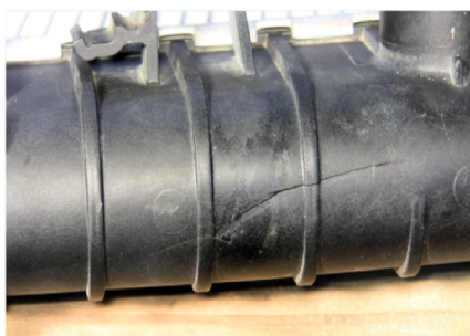
Figure 2.8: ESC in car radiator pipe [12]
