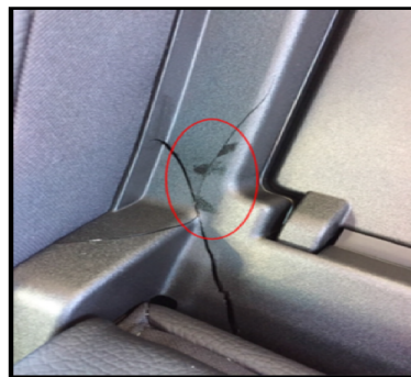
Figure 1.1: ESC occurred in a part of a car
