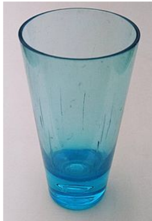
Figure 2.6: ESC in PMMA glass [8]
