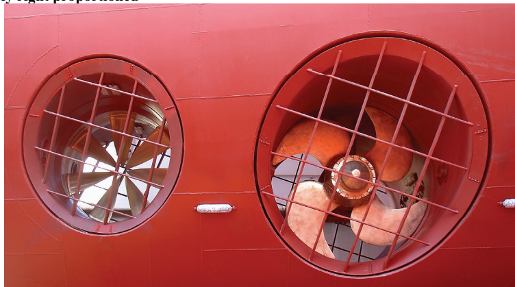
Fig. 56 The pilot RDT mounted in the bow (bulb) on the supply vessel together with a traditional Brunvoll thruster, both with low noise design
