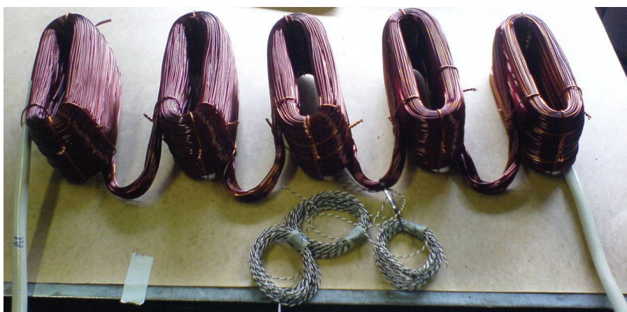
Fig. 109 The coils are wound five and five in series, making up one section
