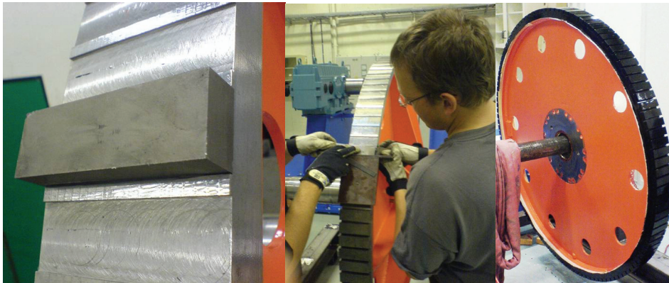
Fig. 111 The mounting of the magnets and painted rotor
