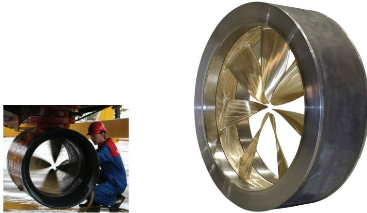
Fig. 55 The prototype RDT (Ø600) [100] to the left and the Brunvoll RDT (Ø1750) [96] to the right, approximately right proportioned
