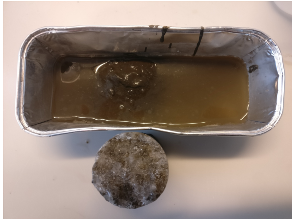
Figure 5.5: Core from 3.3 m in frozen and unfrozen state.
