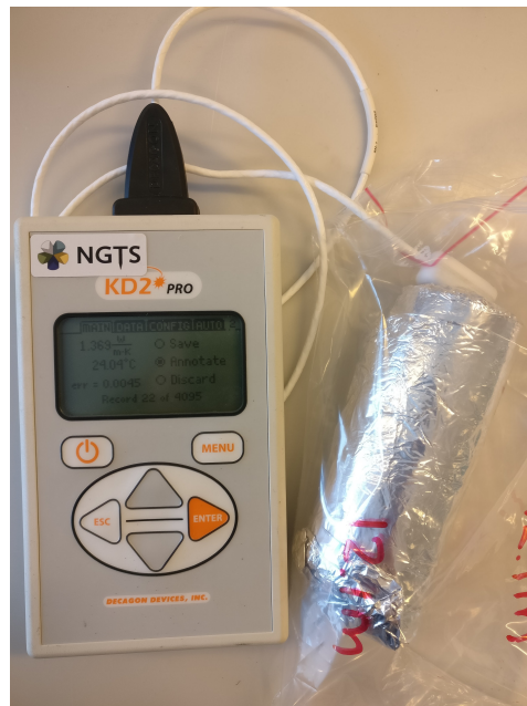
Figure 4.10: Example of experimental setup for the KD2 Pro measurements. This particular sample is taken from a depth of 12.1 meters.
