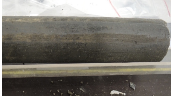
Figure 5.4: Soil sample from a lower layer without large visible ice lenses.
