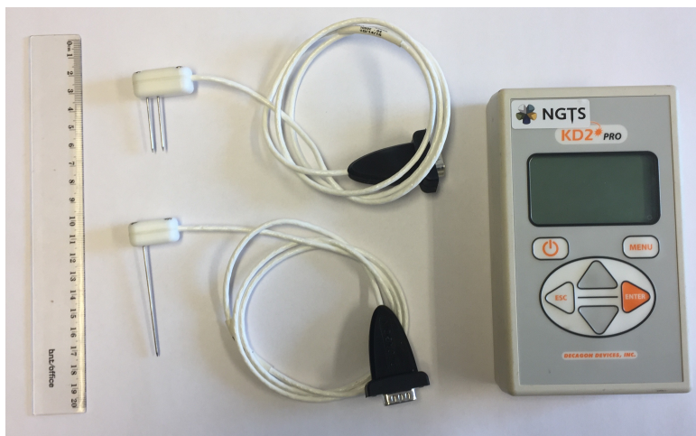
Figure 3.4: The logger and the two needles most appropriate for measuring thermal properties of soil; the SH-1 (dual) and TR-1 (single).
