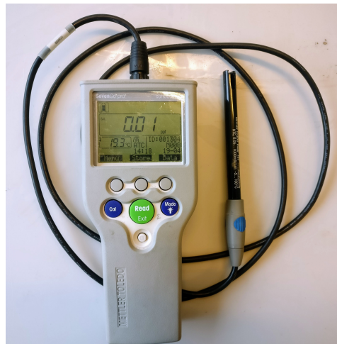
Figure 4.7: Hand-held conductivity meter for salinity measurement
