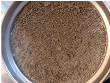
Figure 4.6: Sieving (500 mm) of dried material for organic content determination from 1.3 meter depth. The red-orange colors indicate organic matter. Small pieces of plant material are also visible.
