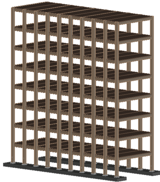
Figure 6.13: Reference building after final decks are mounted.
