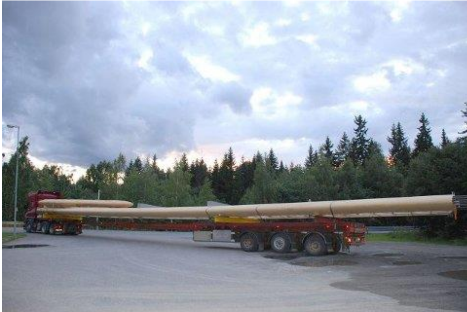
Figure 5.3: Extendable semi-truck loaded with a 33 meter long glulam element (RingerriketBlad, 2008).
