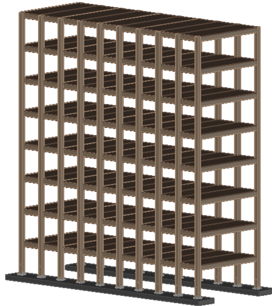
Figure 4.8: Eight story building with strip foundation.
