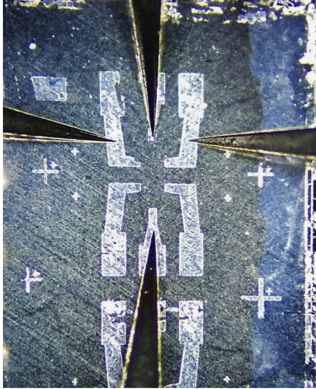
Figure 13: Micromanipulator probe positions for Hall voltage measurements.
