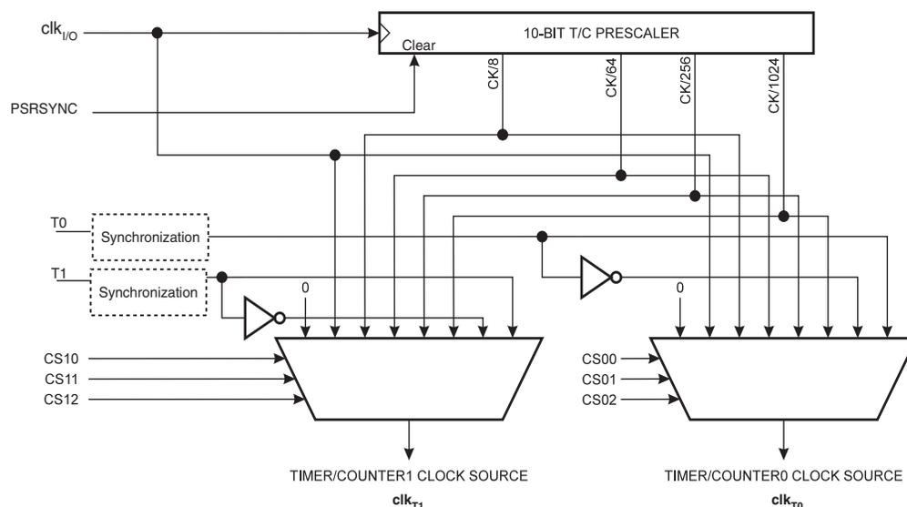
Note: 1. The synchronization logic on the input pins (T1/T0) is shown in [Figure 16-1](#).
