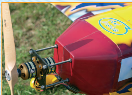
Model EDGE 540 T2 (weight 12,5 kg), with double AXI 5330/20 GOLD LINE
