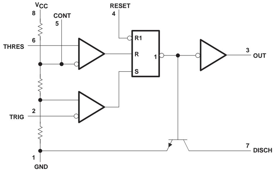
Pin numbers shown are for the D, JG, P, PS, and PW packages.
