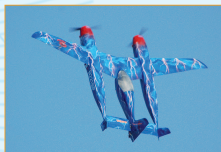
Model Pond Racer (Air-C-Race) with 2x AXI 5345/14 GOLD LINE
