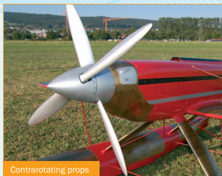
Model EDGE 540 T2 (weight 12,5 kg), with double AXI 5330/20 GOLD LINE
