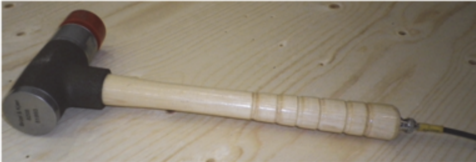
Figure 4.4: Impulse hammer used, picture from "Modal Hammer For Dummies", written by Nathalie Labonnote in 2013
